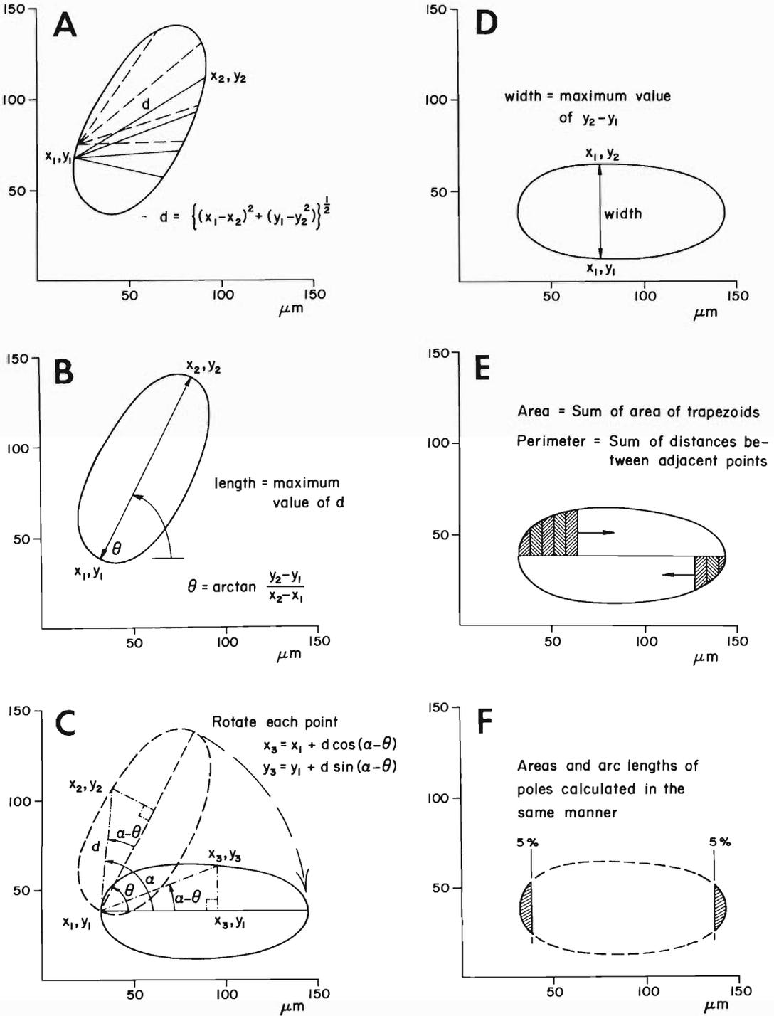
Figure 1. Graphic representation of conversion of coordinate point data into geometric parameters by PARAM, the computer program written by Miles McCreddie. For each egg entered, the computed length, width, area, perimeter, and areas and arc lengths of each pole are stored in a computer file in form suitable for stepwise discriminant analysis.
