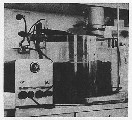
Figure 1. Constant temperature water bath used for incubation and hatching of Nematodirus eggs.
